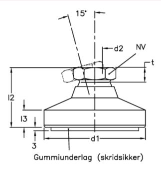
$\begin{array}{lll} d1 & = 40 \\ d2 & = M12 \\ l2 & = 25.5 \\ l3 & = 6.0 \\ NV & = 17.0 \\ Static load (N) = 10000 \\ t min & = 11.5 \end{array}$
